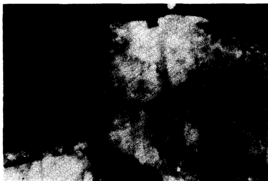
FIG. 8. Microphotograph of a grain of a \text{Te}_2\text{MoO}_7 catalyst after reduction, showing migration of \text{TeMo}_5\text{O}_{16} along reaction paths in the bulk; \times 600 , transparent light.
